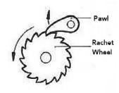
You pull or push the lever and apply the parking brake. The pawl prevents backward movement of either the pedal or lever and, subsequently, the parking brakes are engaged indefinitely.
